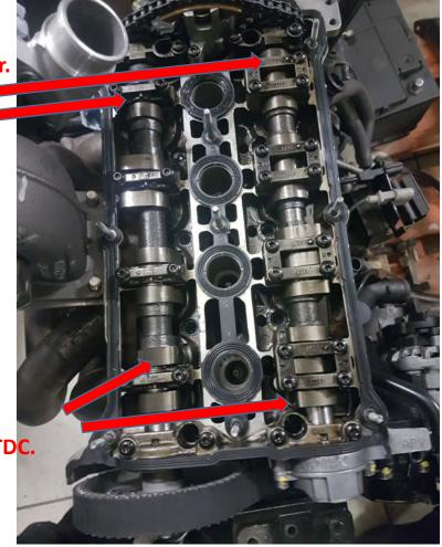
1st cylinder has to be at compression stroke on TDC.
